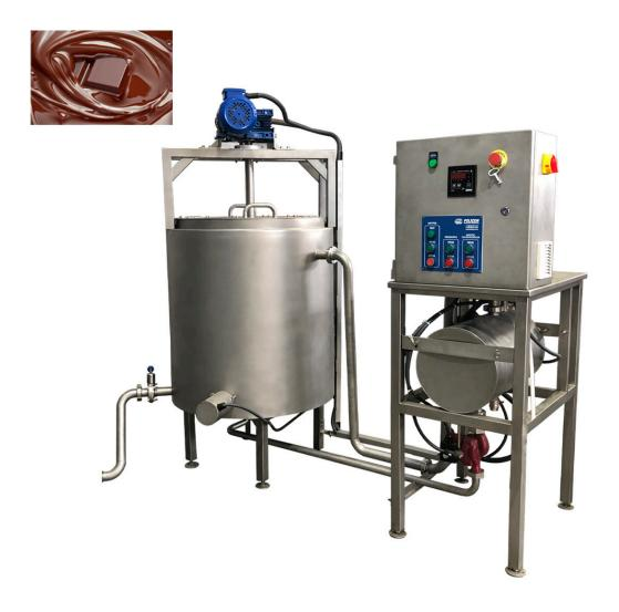
The temperature is maintained by heating the chocolate glaze with a coolant (water) and constant stirring with an anchor-type stirrer.
